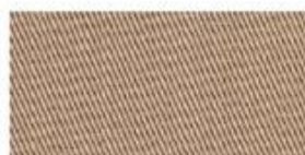
POLY-TWILL Polyester fabric woven with diagonal parallel ridges
