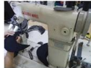
Special Streamlined Lockstitch Machine
